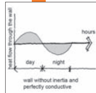
Figure 8.2: Wall and heat flow
